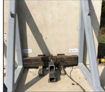
#3 – Shear Test In-Plane/Out-of-Plane
